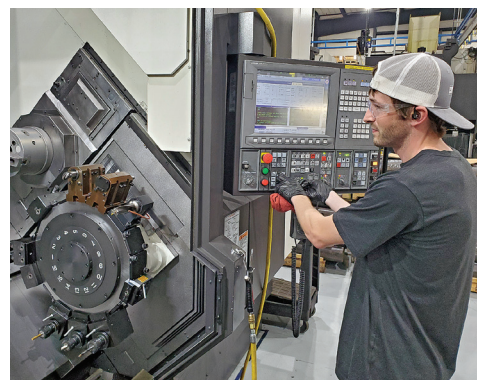
ABOVE: Miles Radovich operates a CNC lathe that is making fan shafts for a large square baler.
